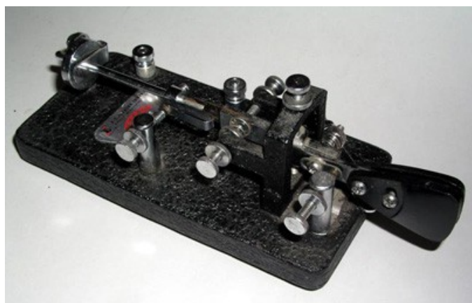
EF Johnson "Speed-X" semi-automatic telegraph key
